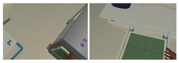
Similarly to the table bucky, the erect detector can be moved up and down. A grid is already inserted but can be removed by pressing the red button.
